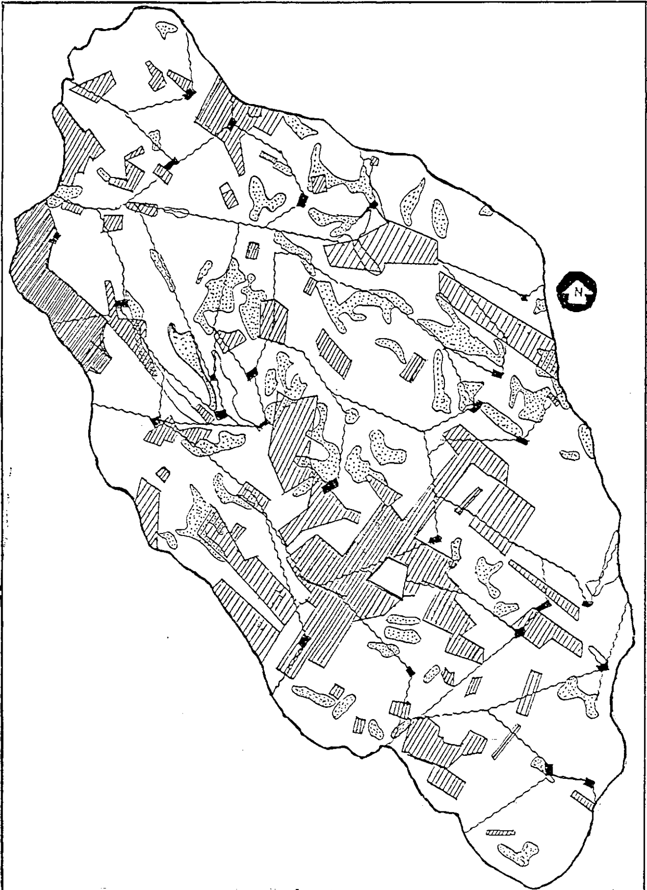
Figure (22) Possible utilized area for range [diagonal lines], land tenure constraints [stippling], dam location [solid black], and water subcatchment [horizontal lines].
