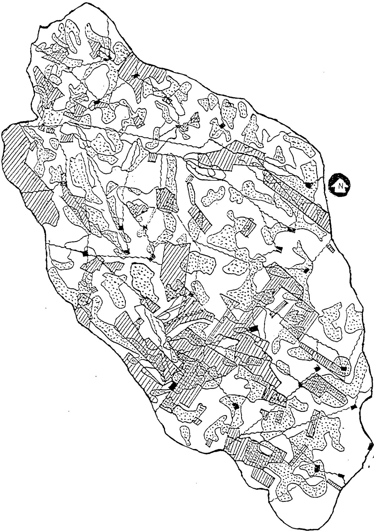
Figure (20): The utilized area of field crops [stippled pattern], land tenure constraints [vertical line pattern], dam location [solid black square], watersubcatchment [irregular outline].
